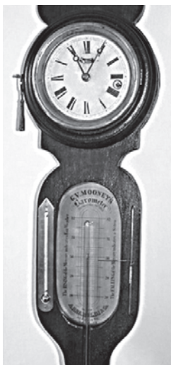
The G.V. Mooney ship barometer (patented in 1865) now in the Society collection.
